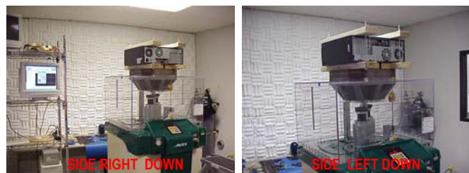
Picture shown is a P172 board with the stiffener installed on a Presario 8000 test platform and setup of the 6 axis.
